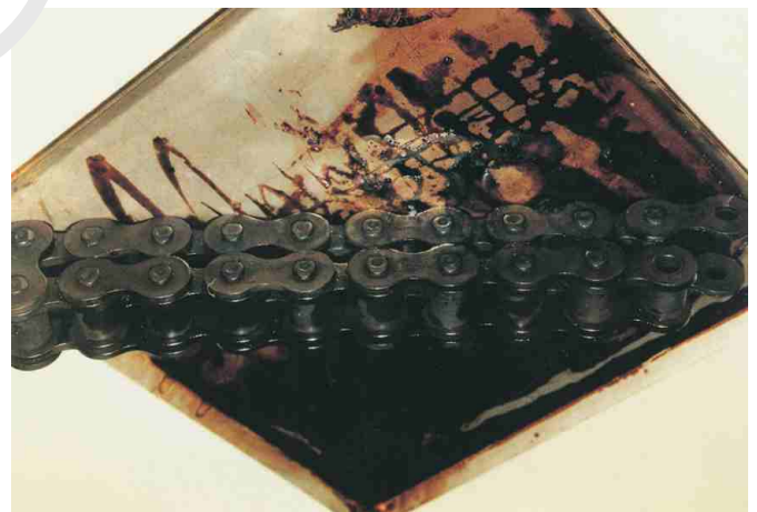
Fig. 2: Roller chain after operation Lubrication with an unfavourable competing oil
